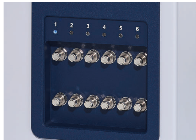
Internal 6-port multiplexer: the operating measurement channel is indicated with a blue LED
