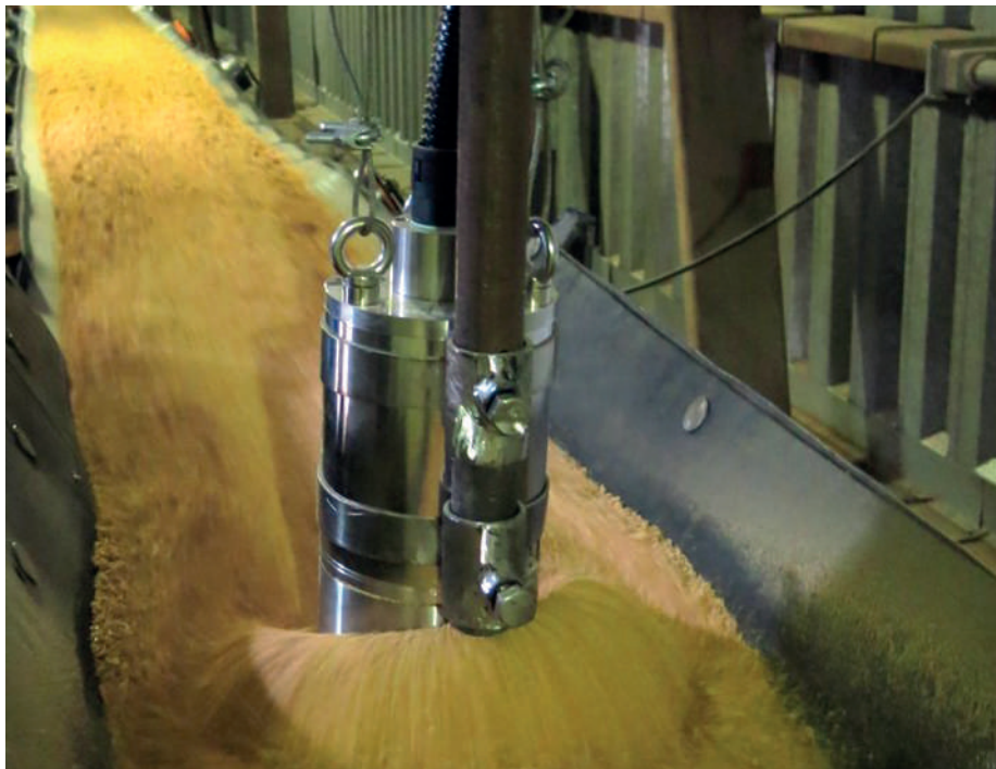
Sensor head mounted over a conveyor belt for the continuous analysis of soybean meal
