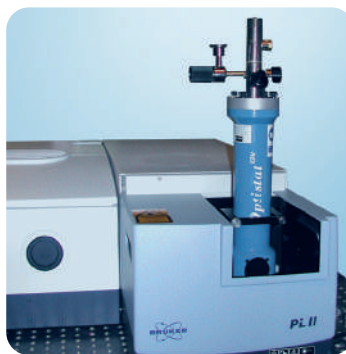
Cryostat adaption for low temperature photoluminescence spectroscopy.
